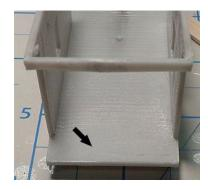
2. Below we did a test on the coupler box (7.95mm) and the coupler box opening (6.09mm). Both sides of the coupler box opening need to be trimmed for the coupler box to fit in the opening.
